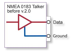
one "NMEA" data line ('**Tx**' '**Data**' or '**Out**'), and used the ground as the other line - similar to a computer serial port. This connection method is referred to as "single ended" instead of the "differential" method used by NMEA 0183 v2.0 devices.
