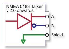
The A is the regular output from the amplifier, and the B is the "inverted" output. The Shield or ground is connected to the talker chassis as shown. In practice, this means line A is zero volts and line B is at 5 volts on an NMEA output when a logical "1" is present,. For a logical "0" line A is at 5 volts and line B is at 0 volts. These voltages would be present only when no load is attached.
